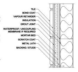
The above installation detail is used with the permission of the Terrazzo Tile & Marble Association of Canada. The installation products shown are Flextile's product recommendations for this specific detail, and are not intended to replace TTMAC's original generic specification.
